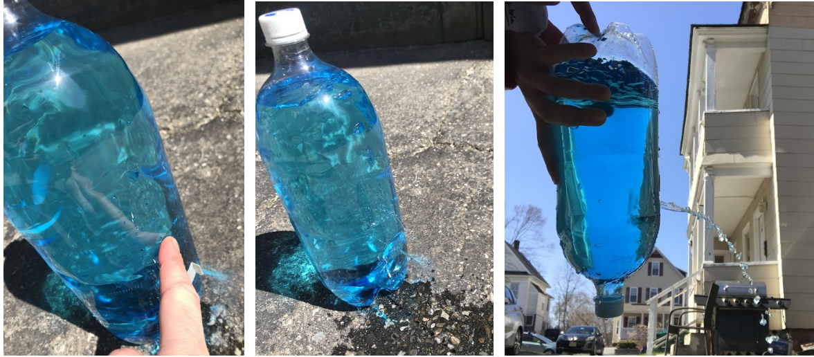
Figure 10 (left): Finger over the second hole. Very slow trickle of water out of the top hole. Figure 10.1 (center): All 3 pieces of tape removed. Water is coming out of the 2nd and 3rd holes (the two nearest the bottom). The lowest hole has a more forceful water flow. Figure 10.2 (right): All three holes open, bottle turned upside down).
