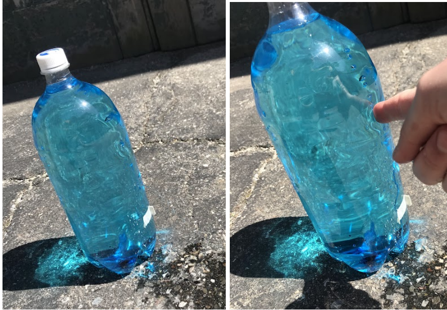
Figure 9 (left): Bottle with the first two pieces of tape removed. Water is coming out of the second hole only. Figure 9.1 (right): Bottle with first two pieces of tape removed and my finger covering the top hole. No water comes out of the second hole.
