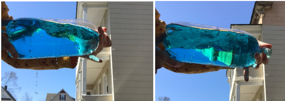
Figure 11 (left): Turning the bottle to horizontal. All 3 holes are still dripping. Figure 11.1 (right): bottle is horizontal, all holes face downward but none are dripping.
